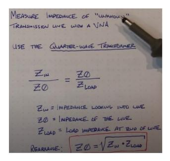
Consider the VNA used to determine the impedance of the unknown coax that is terminated at the far end with 50 Ohms. Using the same formula, knowing 300 Ohms and 50 Ohms, the line impedance = 122.5 Ohms.
