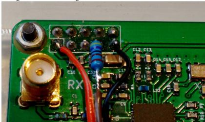
On the picture the red wire is connected to the +3V The Black wire is Ground. The resistor should be a 10K.
