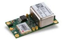
There are several seller that have used these units providing a box and GPS antenna, sold on eBay, note that the active part is second hand, you have no knowledge of how old or what life is left, the problem is that as these age, the oscillator can drift past what the compensation mechanism can adjust, in time the unit will fail due to aging.
