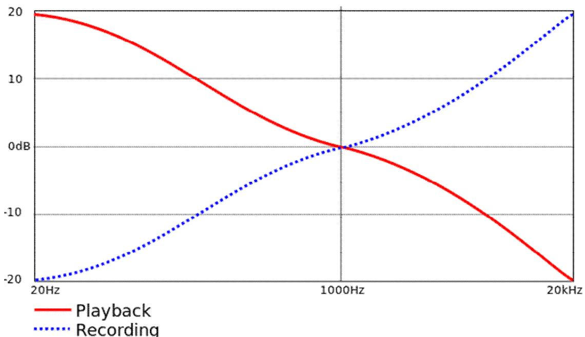
In the case of recording a signal on a vinyl record, emphasis was so devised to overcome the inertia of the cutting head where its more efficient in the low frequencies, hence the
