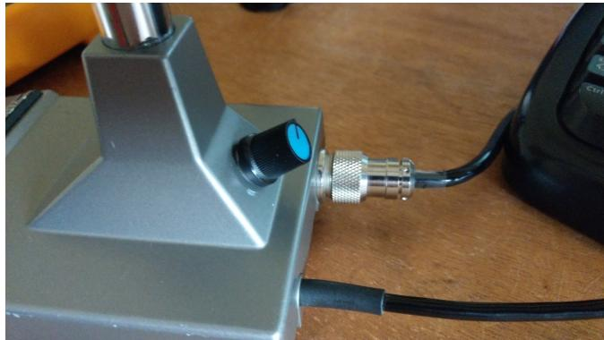
Dress the cable coming from the Microphone head by cutting off the connector, then strip back the wires, the only ones you require are the shielded one. (Ground and Shield)
